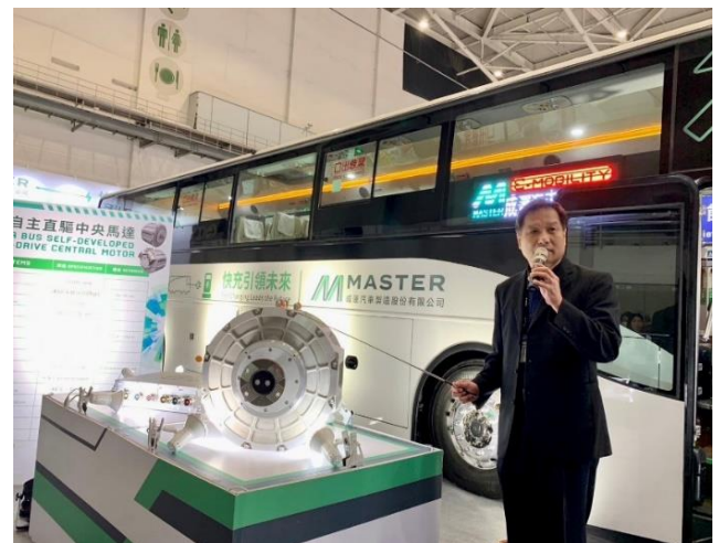
▲ Master Bus President Wu Chung-hsi, introduced Master's self-developed 600hp (450kW) high-power direct-drive central motor, along with the long-distance intercity fast charging electric coach equipped with a 218kWh battery capacity.
